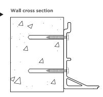
Add washers and lock nuts. Tighten well to fix brackets. Repeat this for all Brackets.
