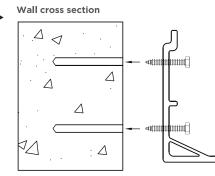
**Insert heavy duty anchors into holes.** (Before inserting locknut and washers.)
