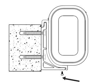
Insert the locking screw on the front of the console and tighten the locking nuts with a hex wrench
